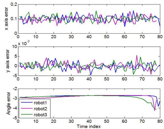
(a) Deviation of coordinates  $x$  and  $y$  and steering angle of three robots.
