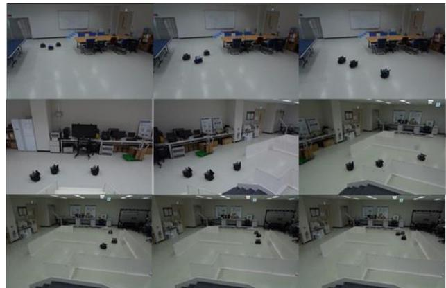
Fig. 9 Composite local path planning of multiple robots in the expanded experiment.
