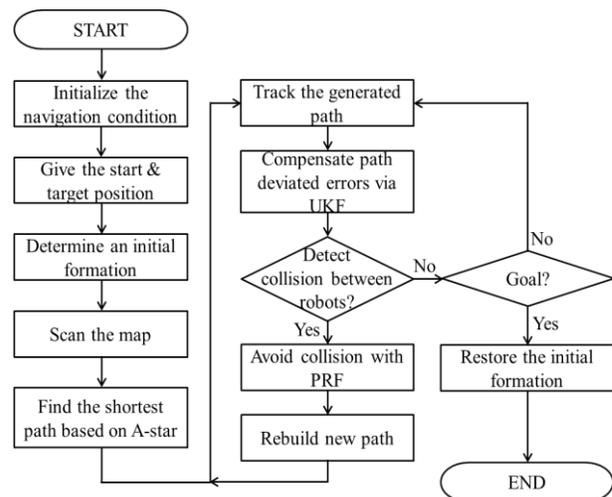
Fig. 1 Flow chart of the composite local path planning.
