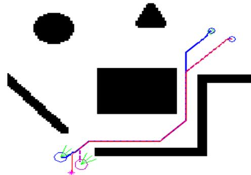
Fig. 2 Navigation for two robots to pass a collision area.
