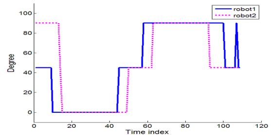
(a) Steering angles of two robots.
