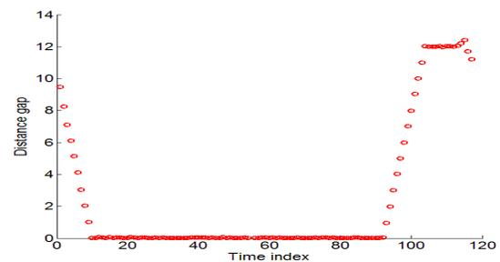
(b) Distance gap between two robots along the original path.
