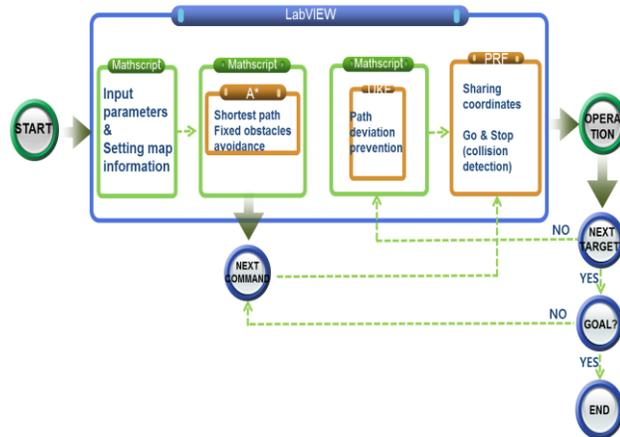
Fig. 6 Operation flow of whole system for experiments.
