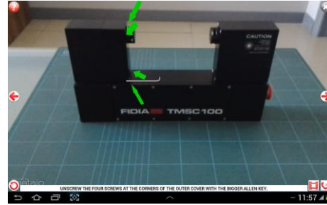
Fig. 3 AR application for maintenance procedures. The application supports the technician through the repair task of an industrial device; textual and 3D assets are shown.
