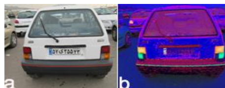
Fig. 3 (a) Entrance image in RGB mode and (b) Image in HSV mode
