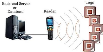
Fig. 1. An architecture of RFID systems [6].
