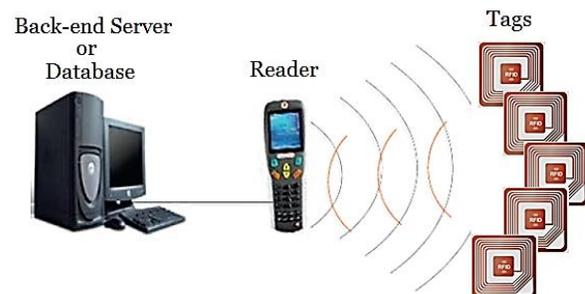
Fig. 1. A System model of RFID systems
