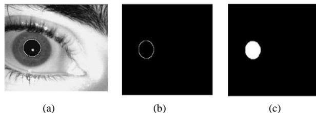
Figure2-5: detecting and recognizing pupil area.
